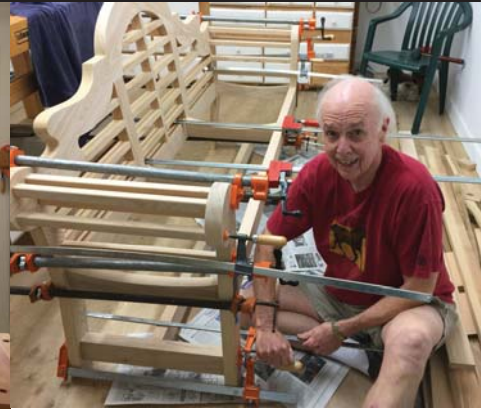
John Altholf finished this cypress garden bench just in time to be used this summer. There are 50 mortise and tenons and over 300 joints! The finish will be an exterior waterseal to protect it from the elements.
