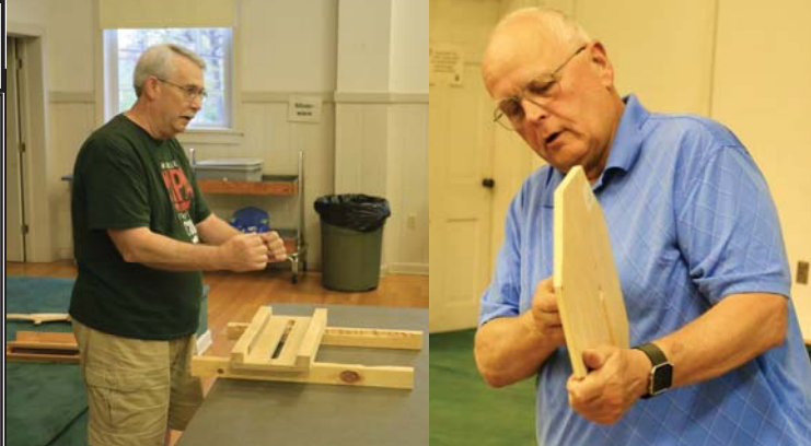
Rob Middleton’s jig is used to flatten glued up boards like cutting boards. The router is moved side to side as the jig is moved fore and aft.
