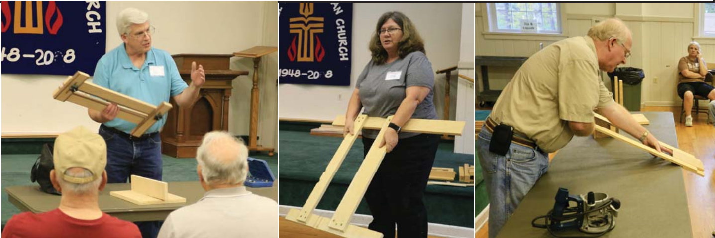
Rich Sherman, Sandy Hansel and Moe Hansen show three different styles of DADO jigs. Rich’s jig is used to rout the dado to the exact width of the piece that goes into the dado. Sandy’s jig is designed to accurately place where you want the dado to be cut. Moe’s jig is used with 2 routers to cut both dovetails and small dados for web frames in case goods.
