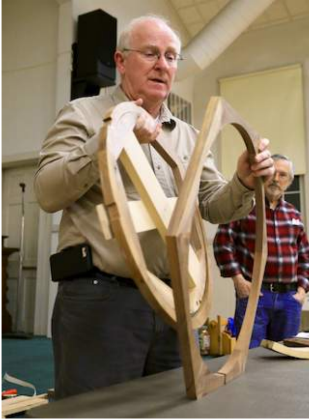
Moe Hansen shows some jigs he used for making his round table.
