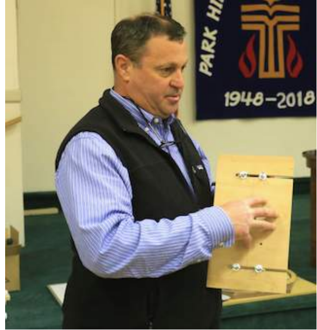
Tom Heutter shows a router jig he made for mortising finger holds in cutting boards.
