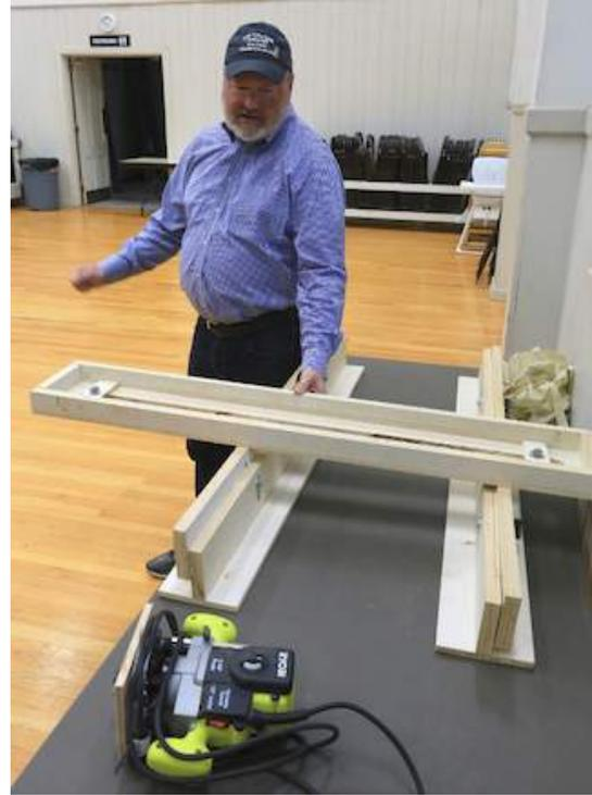
*Bryan Meldrum with a jig he made to use with a router to flatten a live edge slab. He 'locks' the slab in between the two bottom 'rails', places the router in the upper track, then runs the router back and forth across the slab, moving the track down the length of the slab.*
